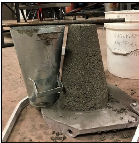
Figure 1: Example of Slump Test Performed
